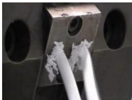
Control: 61% ATH, 0% Dow Corning 4-7081 Resin Modifier
